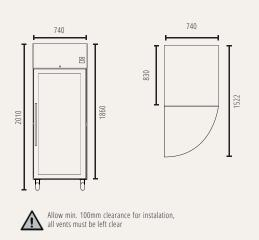
Temperature set range : -2°C to +8°C Gross/net weight: 147/132 kg Energy consumption in 24h: 3.1 kWh
